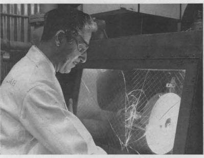
CRACKS IN SAFETY GLASS looked like lucky stars to Tom Dadian (8115-1) recently at the Livermore Laboratory. The 1/4-inch thick glass stopped a fragment of a broken wheel thrown by an abrasive cutoff wheel in the metallurgical lab. The machine has since been equipped with a metal wheel guard to limit hazards.
